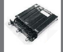
External Duplexer DT01 (Freq. Range: 137-172MHz, Tx/Rx Split: 4-15MHz)
