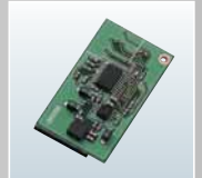
UT-124R Man down unit. Automatically sends an emergency signal when the transceiver is left in a horizontal position for a preset time.
