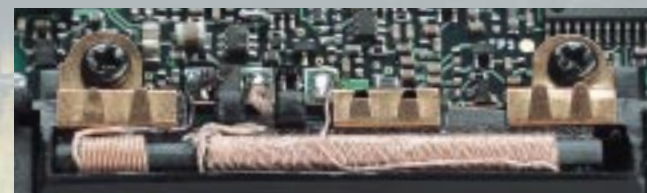
Internal ferrite bar antenna
