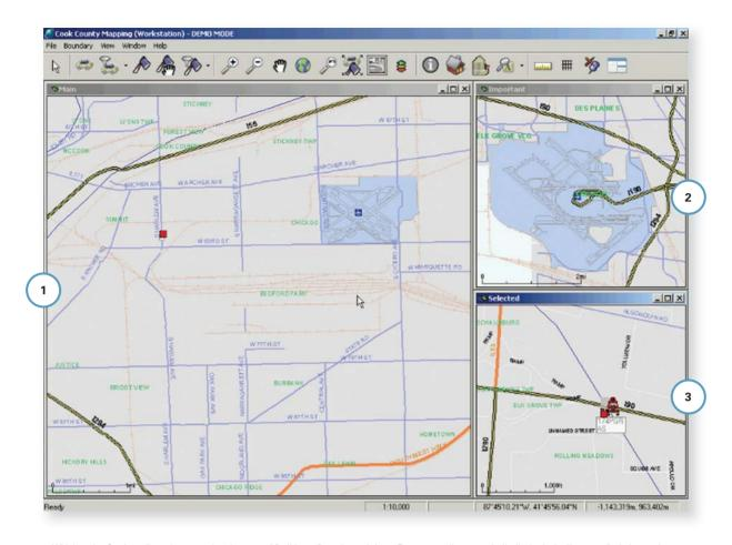
With Location Services, dispatchers can take advantage of flexible configuration and views. Emergency calls automatically display in the "Important" window, and remain on the screen until dismissed by the dispatcher.
